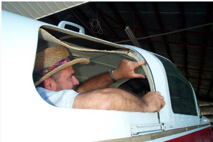
Cleaning up a read window frame during the hands-on maintenance demos.
