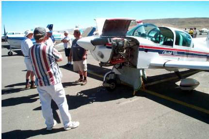
Scott Jernigan's plane is propped up on a sawhorse in preparation for the removal of the nose strut as part of the hands-on maintenance demo.
