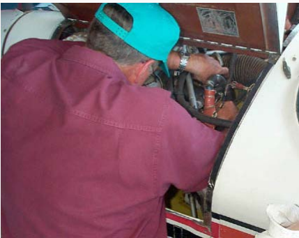
David Fletcher reaches in to secure the screen housing as part of the oil change hands-on maintenance demo.
