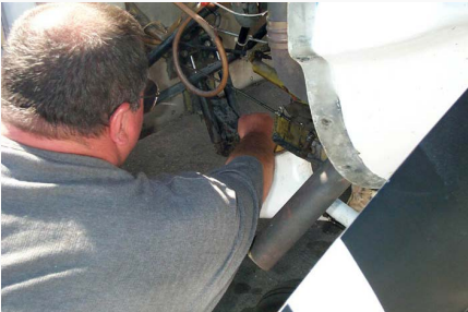
Scott Jernigan prepares his plane's nose strut for removal as part of the hands-on maintenance demo.
