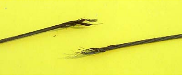
Mark's broken rudder cable.
