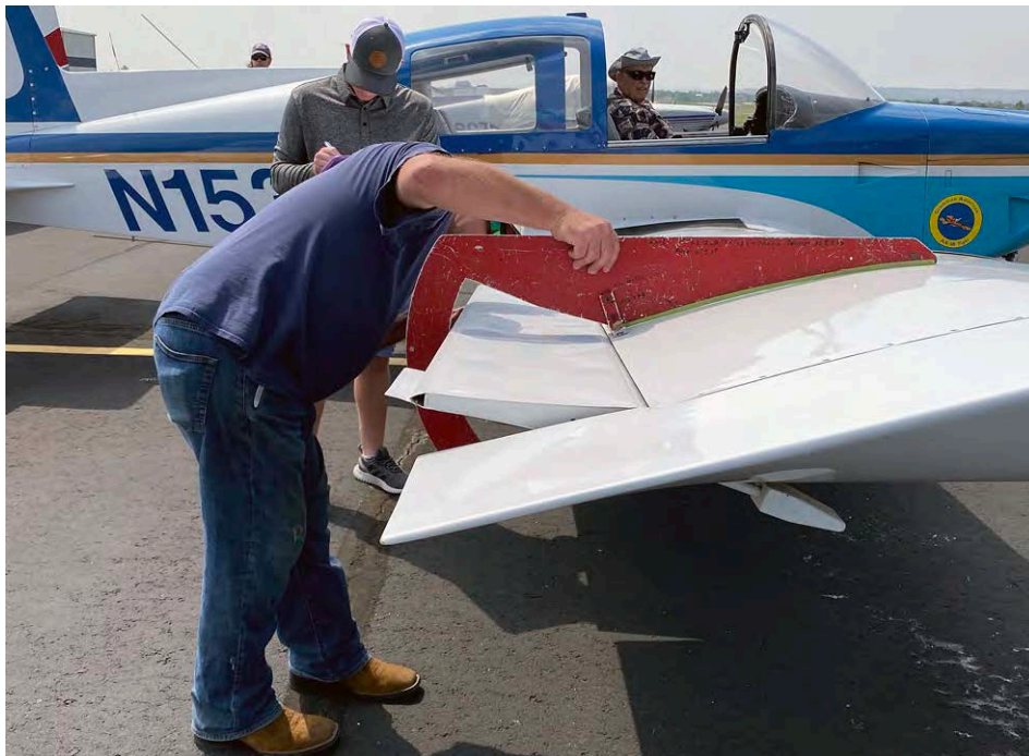
A couple of David Fletcher's techs are over doing rigging checks.
