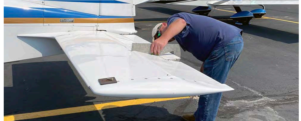
A couple of David Fletcher's techs are over doing rigging checks.
