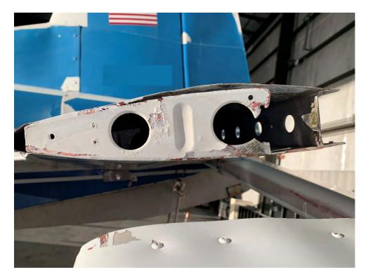
Figure 1. Severely Damaged Horizontal Stabilizer with Skin Delamination and Indications of Bondline Corrosion, Model AA-5
